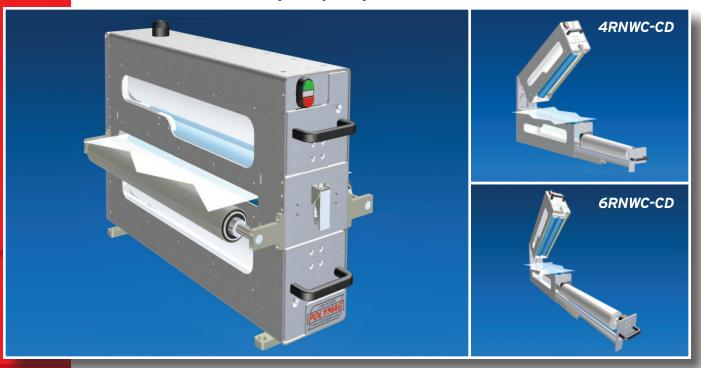
Two-sided, contact web cleaning for "Continual Run," "Stop & Go" or "Limited Access" applications including slitters, coaters, die-cutters, laminators, presses, embossers and more. Sturdy, 12 gauge stainless steel and anodized aluminum constructed "clamshell" design for easy CCR maintenance and web thread-up. Drawer slides promote "on-the-fly" tape change capability. LED window lighting provides easy CCR and tape roll visibility and flashing operator alarms for tape change.
