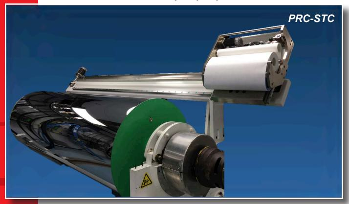
Wide, fabric-covered, touch roll cleaning head performs zonal steps during a quick, traversal cleaning of the rotating process roll surface. Fabric is refreshed at each step completion via an unwind/rewind system on the cleaning head.
