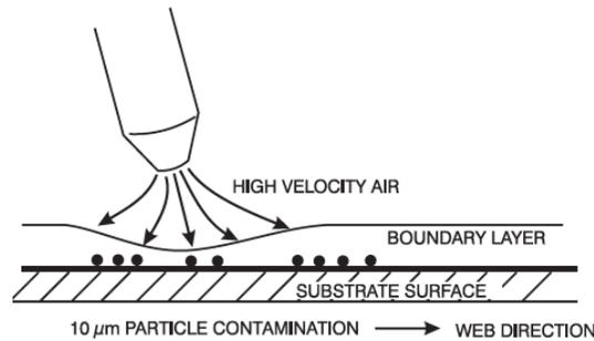
**Figure 1: Typical air knife/vacuum systems**
