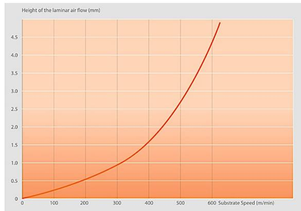
**Table 2: Height of laminar air flow with respect to substrate speed<sup>7</sup> (Hildebrand, 2017)**
