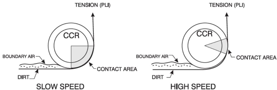
**Figure 2: Contact area with respect to speed**
