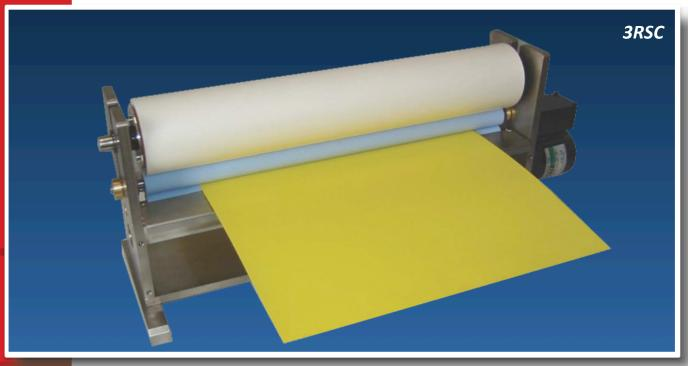
The Polymag® Tek Two-Sided, 3 Roll Sheet Cleaner (3RSC) offers customized sheet cleaning to meet your most unique needs. Driven Contact Cleaning Rolls (CCRS) remove contamination from the sheet and then transfer contamination to an adhesive tape roll. The CCRS continue to rotate in between sheet feeding, cleaning each other and transferring contaminants to the adhesive tape roll for permanent removal.
