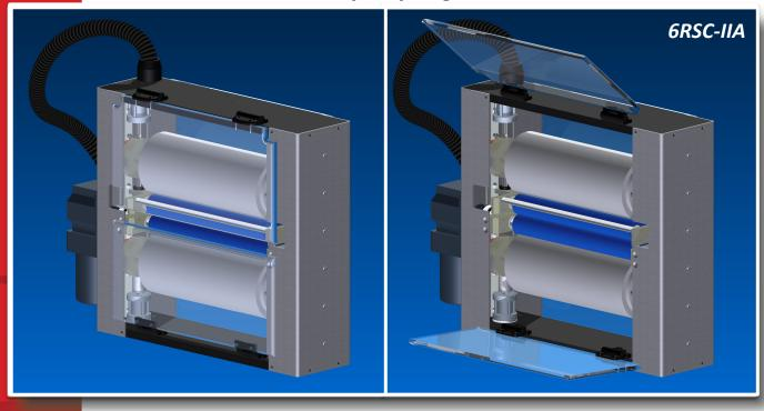
Polymag® Tek Two-Sided, Sheet Cleaner (6RSC-IIA) offers customized sheet cleaning to meet your most unique needs. Driven Contact Cleaning Rolls (CCRS) remove contamination from the sheet and then transfer contamination to Adhesive Tape Rolls. Custom in-feed and exit conveyers are available to establish the most efficient sheet cleaning processes.
