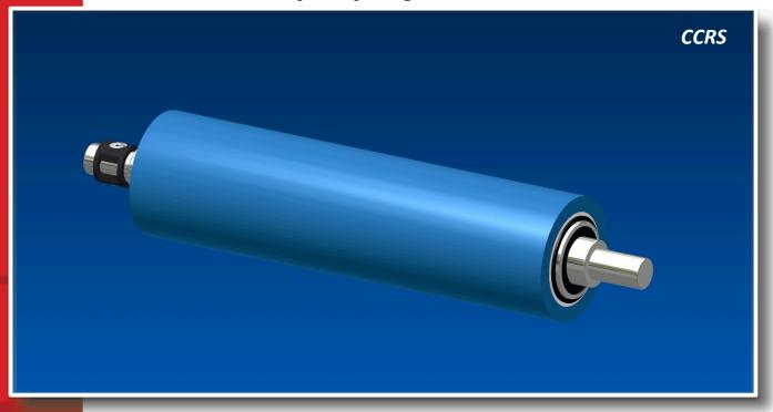
Polymag® Tek Blue-S™ Contact Cleaning Rolls efficiently clean your substrate through continual contact, breaking through the boundary layer of air to capture loose particulate, dirt and debris. The high surface energy of the Blue-S™ Polymeric material attracts and holds contaminants until they can be transferred to an adhesive tape roll for permanent elimination.
