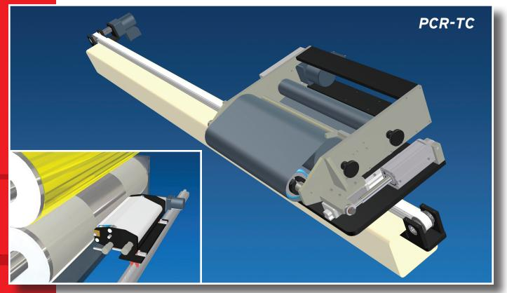
Wide, fabric-covered, touch roll cleaning head performs a quick, traversal cleaning of the rotating process roll surface. Fabric is refreshed during the traversal movement via an unwind/rewind system on the cleaning head.
